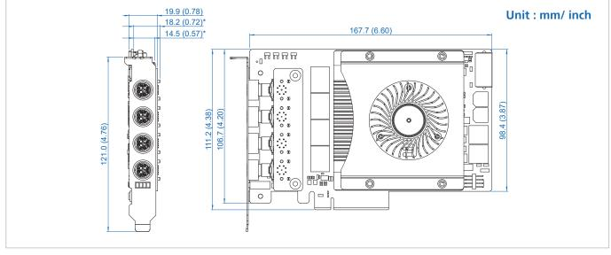
\*PE-7004MX is slightly thicker than the standard PCIe card width (14.5mm) and may interfere with the slot on the right side. For mechanical assessment, please contact the Vecow team.
